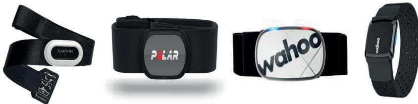
Figure 2. Arm and chest heart rate bands with Bluetooth capability that provide ANT+ data transfer. (Garmin, 2023; Polar, 2023; Wahoo, 2023)
