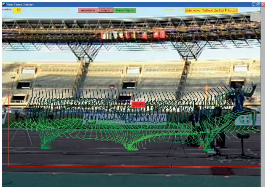
Figure 10. Stickfigure imposed on a field of the video used to conduct the 2D-DLT analysis using the K-Motion v.15 software (Kinvent, Orsay, France).
