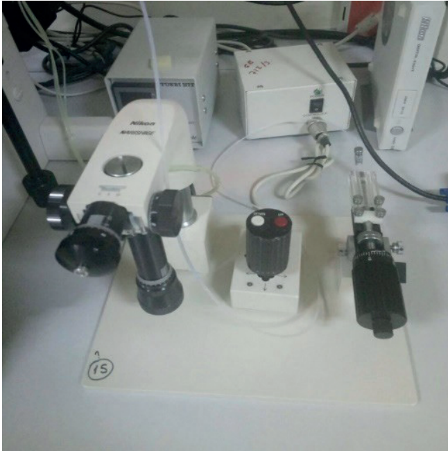
Figure 5: Hydraulic micromanipulator control panel
