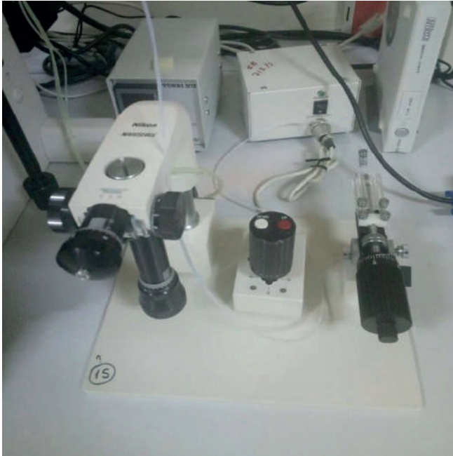
Figure 5: Hydraulic micromanipulator control panel
